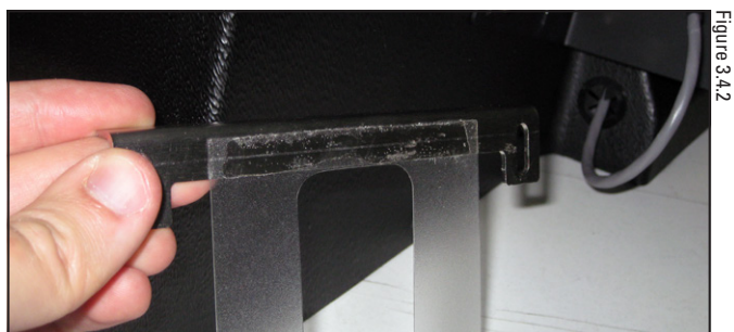
Change the mylar ticket deflector and re-attach the metal film retainer
