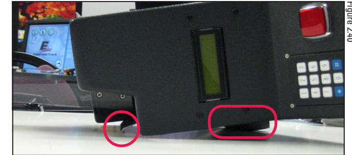
The 2 support points when the ticket counter is laying on its side
