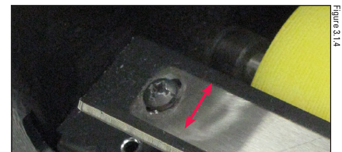
Move the metal ticket guide back and forth for a more precise adjustment
