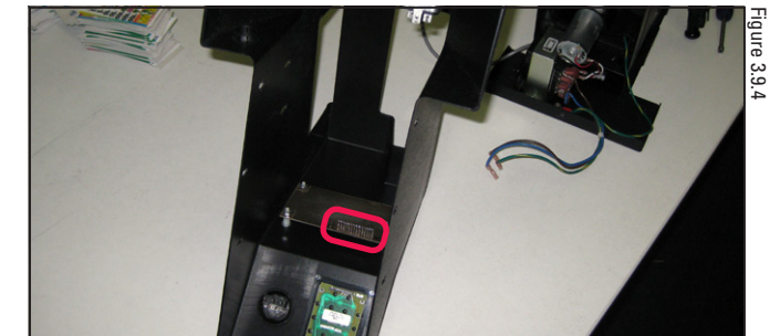
Oriented in this manner, it is easier to perform maintenance on the LCD assembly
