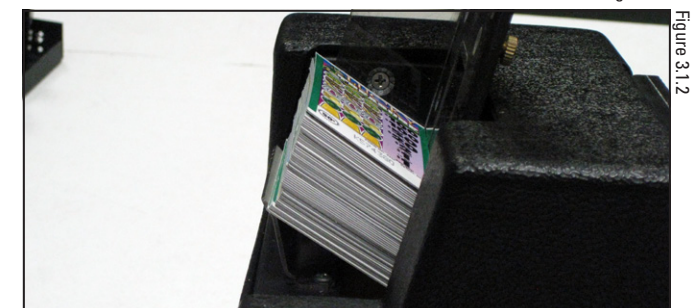
The metal ticket guide is too close to the column
